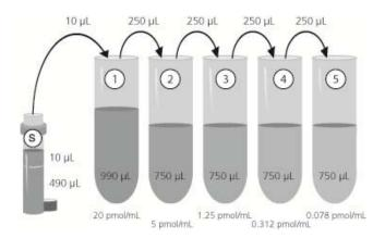
Allow the 2,000 pmol/mL standard stock to warm to room temperature. Label five 12mm x 75mm tubes #1 through #5. Pipet 990 µL of the appropriate sample diluent into tube #1. Pipet 750 μL of the appropriate sample diluent into tubes #2 through #5. Add 10 µL of the 2,000 pmol/mL standard stock into tube #1 and vortex thoroughly. Add 250 μL of tube #1 to tube #2 and vortex thoroughly. Add 250 μL of tube #2 to tube #3 and vortex thoroughly. Continue this for tubes #4 through #5.
