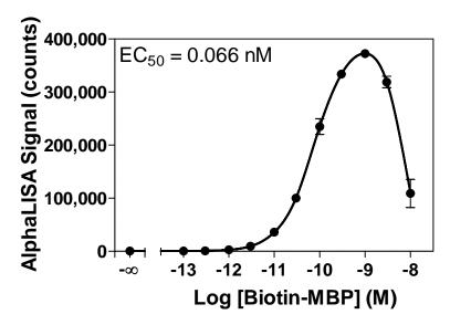
Titration assay using the Quality Control protocol. Signal was detected with an EnVision Alpha instrument 2102.
