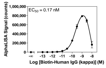
Titration assay using the Quality Control protocol. Signal was detected with an EnVision Alpha instrument 2102.
