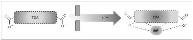
Figure 2. Detection of the released ligand. After addition of EU3+-solution to the sample a fluorescent chelate is formed.
